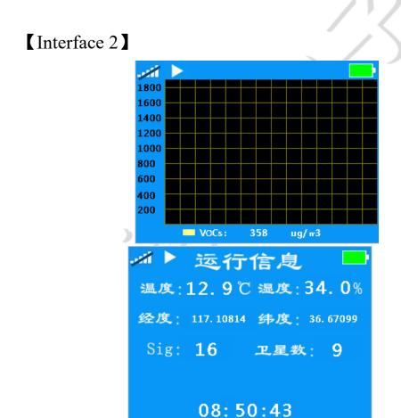
Press the "Switch key" to switch to display the real-time VOCs concentration curve and other operating information of the
