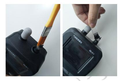
Step 4: After cleaning the air inlet and the filter screen, assemble the gas sampling probe and reinstall it on the device. Pay special attention to ensure that the two ends of the black silicone sealing tube are tightly installed with the filter screen and the sensor inlet respectively.
