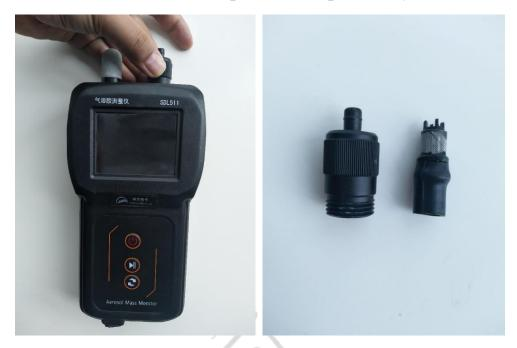
Step 2: Clean the air inlet with an awl needle to ensure that the air inlet is unobstructed and free of foreign objects.
